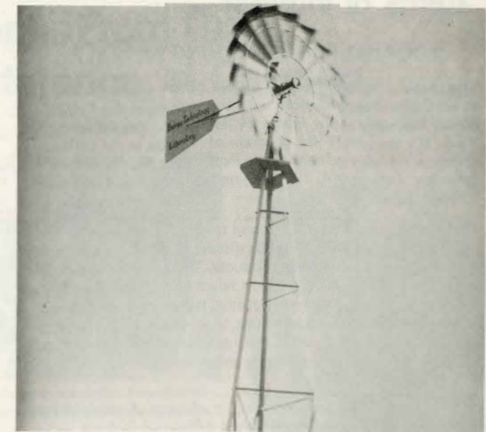
The completely reconditioned 8' diameter water pumping windmill. Students spent their summer vacation in the Energy Technology Lab to complete the work.
