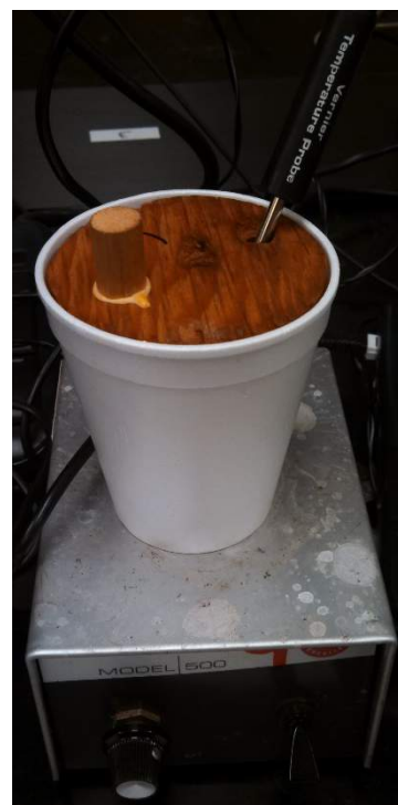
Figure 1: Coffee cup calorimeter setup
