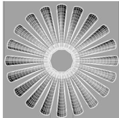
Figure 11 Top View showing internal decagonal tube
