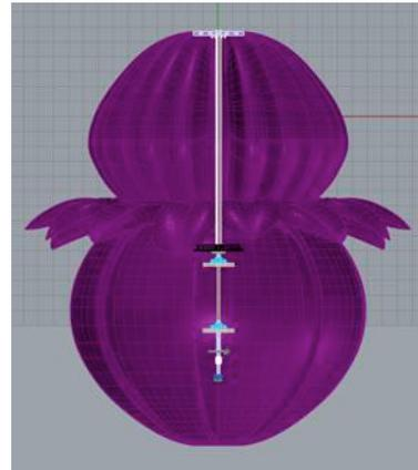
Figure 13 Digital model introducing Savonius wind turbine mechanism, to rotate the top piece
