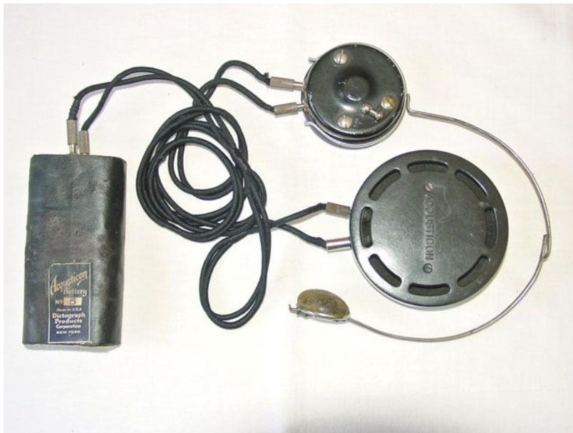
Bell made possible electronic amplified sound with a carbon microphone and a battery. These hearing aids were cumbersome boxes containing visible wires and a heavy battery that lasted only a few hours, and worn around the neck. Sometimes, “battery packs” were worn on
