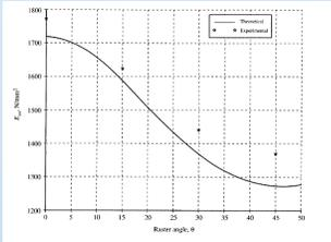
Filament angle vs. Modulus [2]
