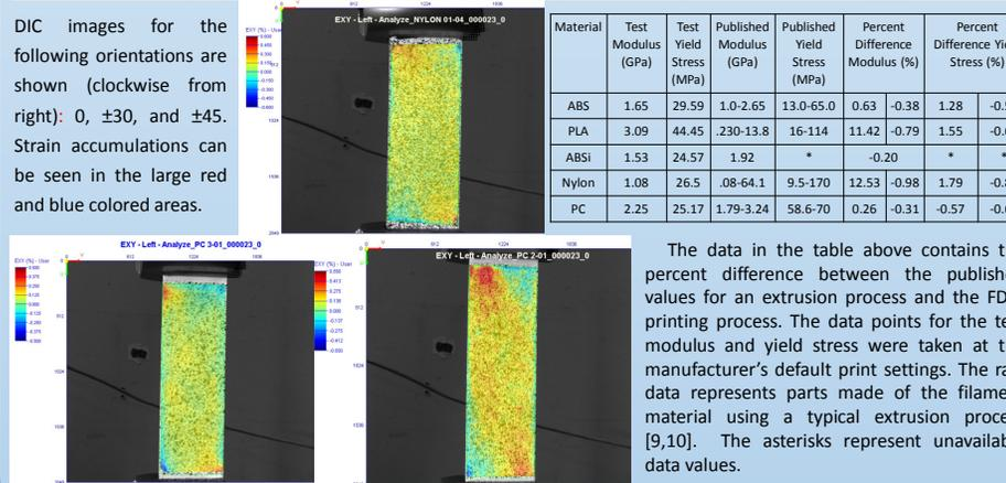
The data in the table above contains the percent difference between the published values for an extrusion process and the FDM printing process. The data points for the test modulus and yield stress were taken at the manufacturer's default print settings. The raw data represents parts made of the filament material using a typical extrusion process [9,10]. The asterisks represent unavailable data values.
