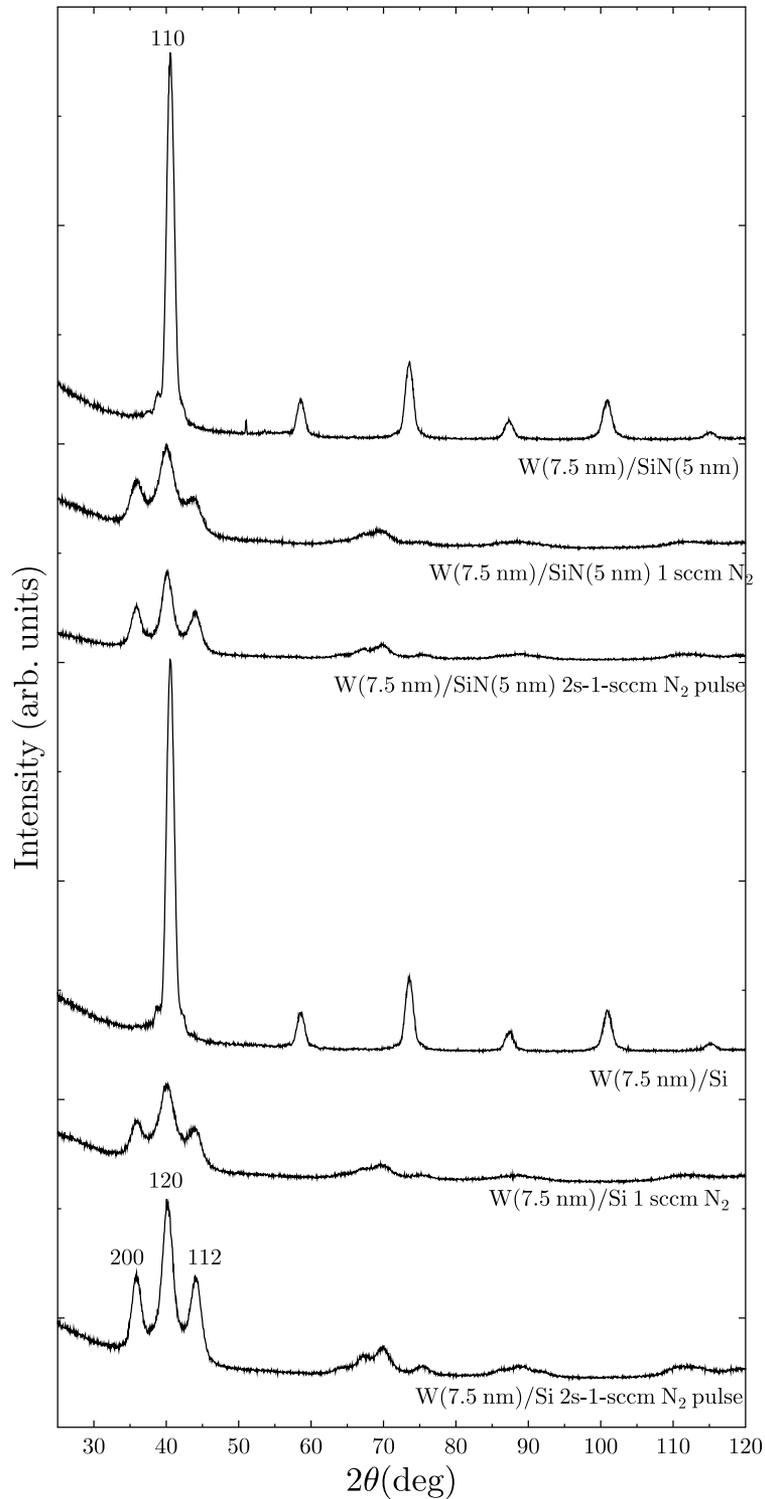
FIG. 2. X-ray diffraction patterns of the 7.5 nm W films deposited on the substrates as indicated.
