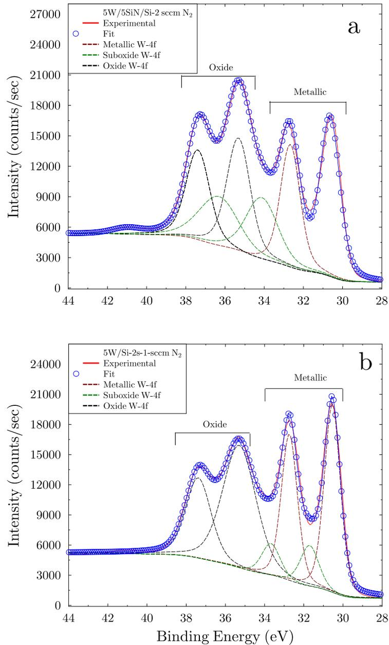
FIG. 4. a.) X-ray photoelectron spectroscopy result of 5 nm amorphous-like W film. b.) X-ray photoelectron spectroscopy result of 5 nm  $\beta$ W film.
