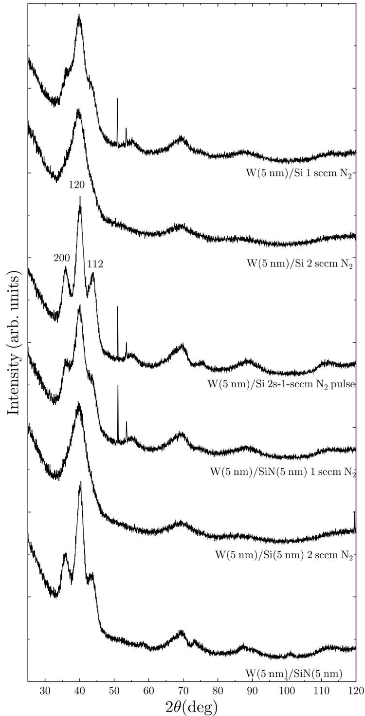
FIG. 1. X-ray diffraction patterns of the 5 nm W films deposited on the substrates as indicated.
