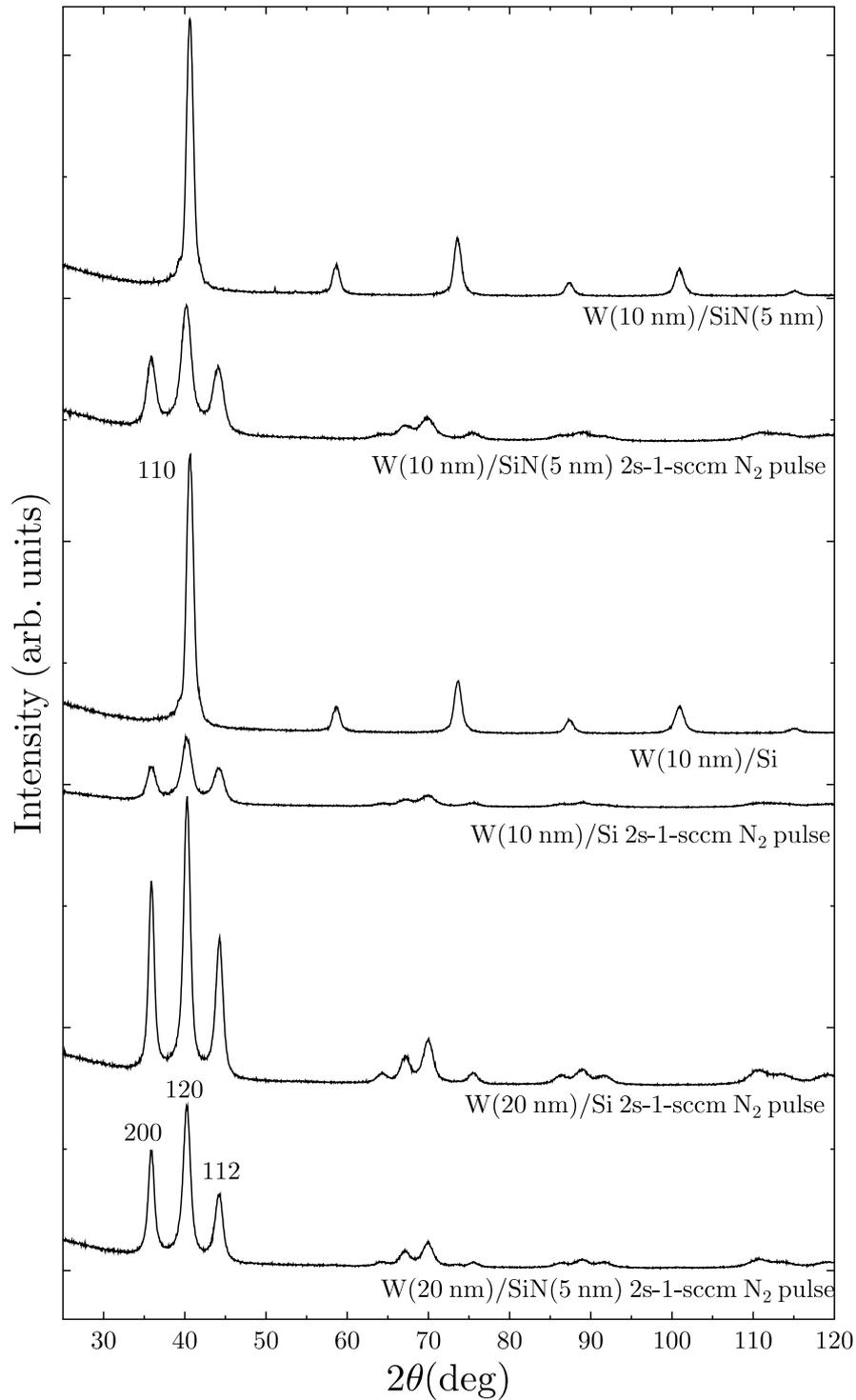
FIG. 3. X-ray diffraction patterns of the 10 nm and 20 nm W films deposited on the substrates as indicated.
