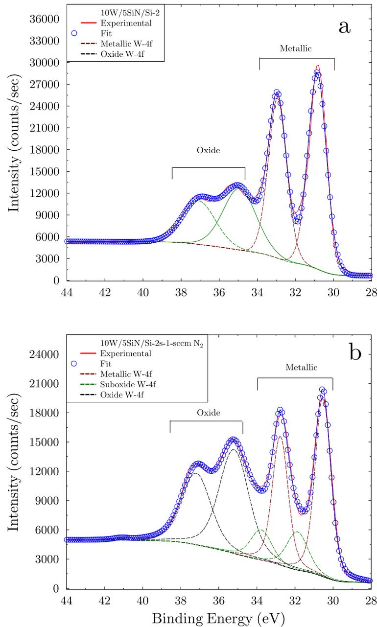
FIG. 5. a.) X-ray photoelectron spectroscopy result of 10 nm  $\alpha$  W film. b.) X-ray photoelectron spectroscopy result of 10 nm  $\beta$ W film.
