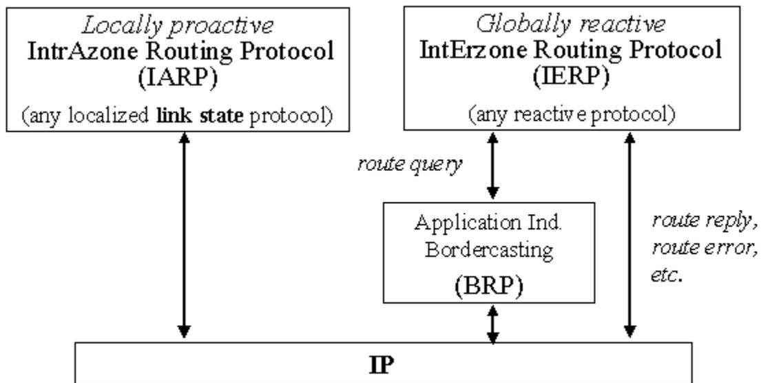
Figure 7: Zone Routing Protocol Architecture<sup>[4]</sup>
