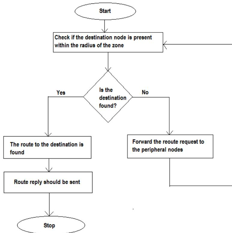
Figure 8: Route Discovery Process Explained Using A Flowchart <sup>[9]</sup>
