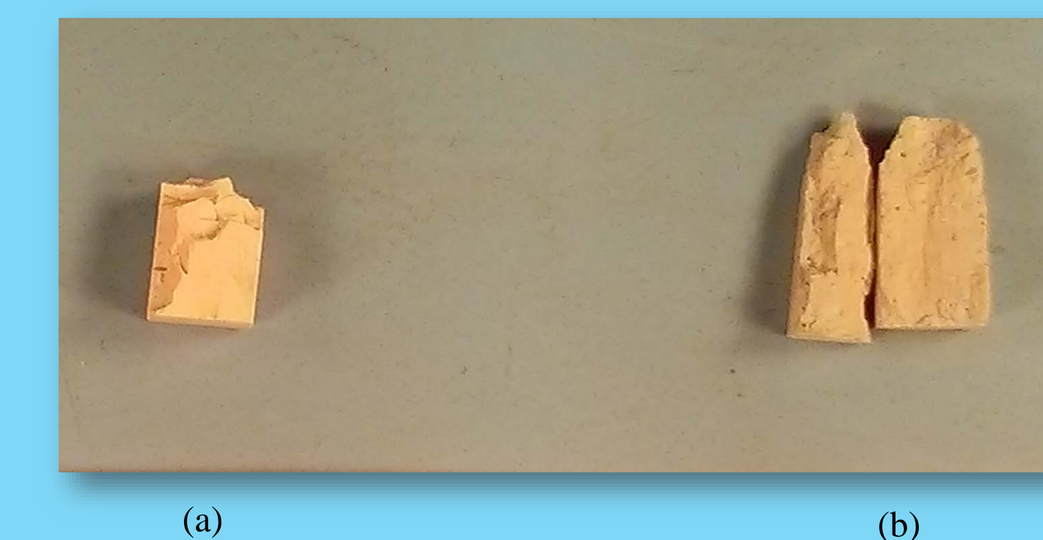
Fig. 7 Post compression test (a) Neat Geopolymer and (b) Geopolymer with 4 wt% RHA and SCW
