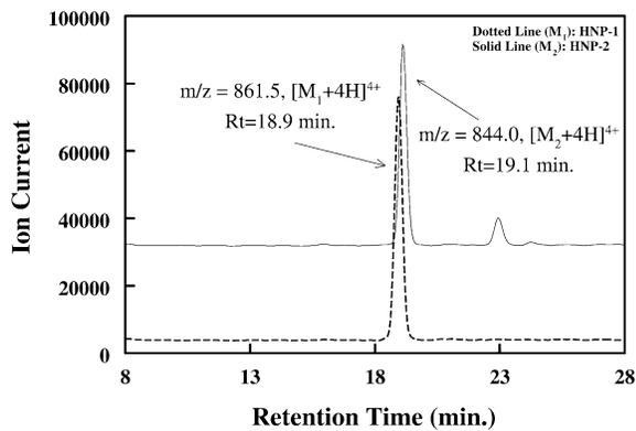
**Figure 7.** Selected-ion recording (SIR) chromatograms of HNP-1 (dotted line) and HNP-2 (solid line) from a human tear sample. The quantification of HNP-1 ( $m/z = 861.5$ ) and HNP-2 ( $m/z = 844.0$ ) was based on peak areas from the SIR chromatograms.
