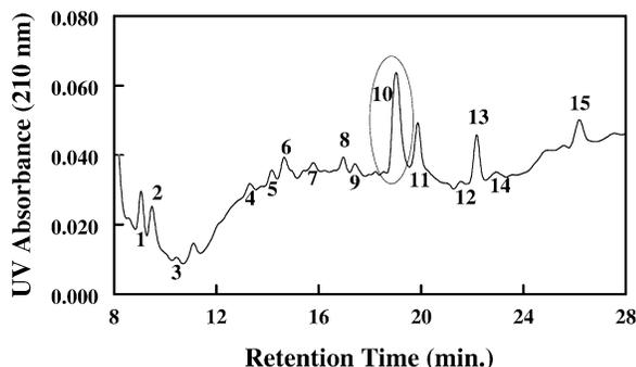
**Figure 4.** HPLC–UV chromatogram of a typical human tear sample. Magnified chromatogram in the region of 8 to 28 min revealed a complex elution pattern. As detailed in the results, peak 10 was shown to contain human  $\alpha$ -defensins, HNP-1, HNP-2 and HNP-3.
