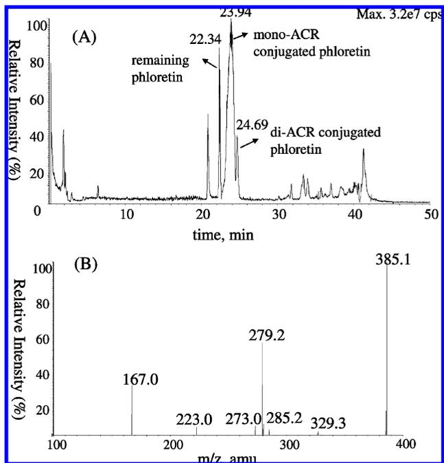
**Figure 6.** Total ion chromatogram of the reaction products in the incubation of phloretin and ACR together (A). MS/MS spectrum of the precursor ion of  $m/z$   $[M - H]^-$  385.1 as diACR-conjugated phloretin (B).
