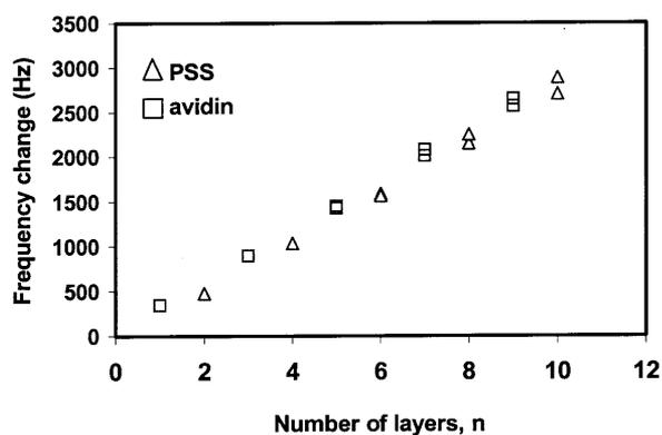
Fig. 3. QCM frequency change for the construction of alternating avidin/PSS multilayer films formed on the (PAAH/PSS) precursor film on 3',3'-dithiopropionic acid modified electrodes. The odd layer numbers correspond to avidin deposition and the even layer numbers to PSS. Experimental data points for two separate experiments are shown.
