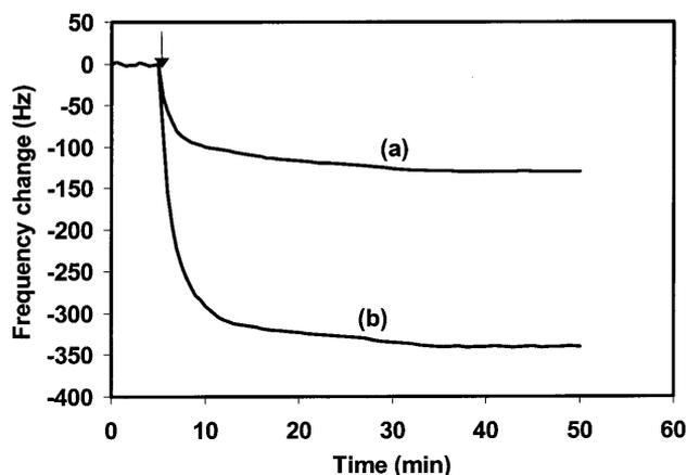
Fig. 2. QCM frequency change as function of time for the immobilization of avidin from 0.1 mg/l aqueous avidin solution: (a) avidin binding to 3',3'-dithiopropionic acid/EDC monolayer; (b) avidin adsorbing electrostatically on the outer negatively charged PSS layer of the (PAAH/PSS) precursor film. The arrow indicates the time at which avidin was injected into water solution.
