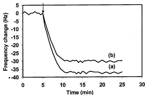
Fig. 5. QCM frequency change versus time for the immobilization of: (a) DNA probe having disulfide group on the QCM electrode by chemisorption from aqueous solution (sensing film 6); (b) DNA probe immobilized on the PAAH/PSS/PAAH precursor film by electrostatic adsorption (sensing film 4).
