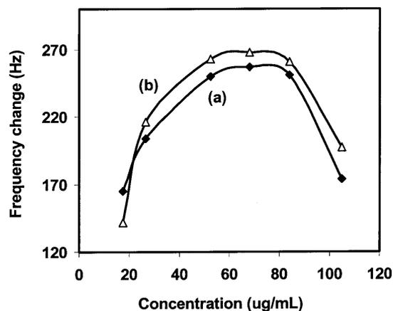
Fig. 7. Effects of target DNA concentration on sensor response. Hybridization was conducted on 0.05 M HEPES buffer solution with 0.5 M NaCl.
