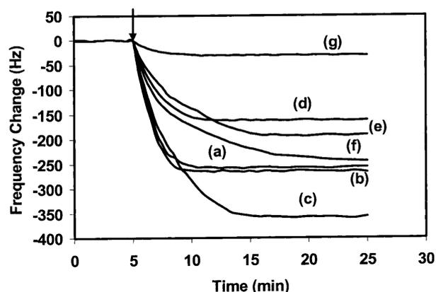
Fig. 6. Frequency change versus time for the hybridization experiments on QCM sensor with different sensing films in HEPES buffer solution of  $52.5 \mu\text{g/ml}$  41/42 $\beta$  DNA: (a) sensing film 1; (b) sensing film 2; (c) sensing film 3; (d) sensing film 4; (e) sensing film 5; (f) sensing film 6; (g) hybridization on sensing film 1 with  $58.75 \mu\text{g/ml}$  of 41/42N DNA. The arrow indicates the time at which the target PCR product was injected into water solution.
