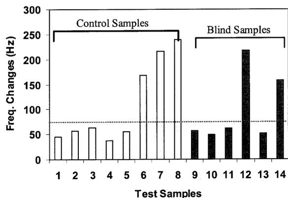
Fig. 8. Classification of positive and negative samples by QCM sensor coated with sensing film 1.
