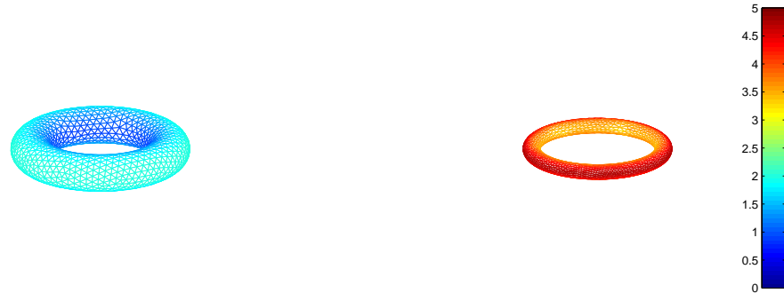
Figure 7.4: The evolution of a closed torus mesh (major radius = 1.0, minor radius = 0.25) under mean curvature flow using our semi-implicit method. The colormap reflects the mean curvature. (left) surface before evolution. (right) surface after 0.09 seconds of evolution.
