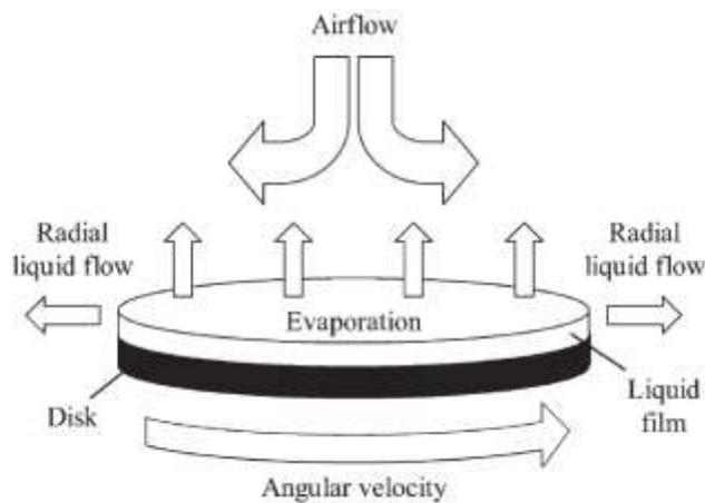
Figure 0-1 Scheme of the spin coat process [4]
