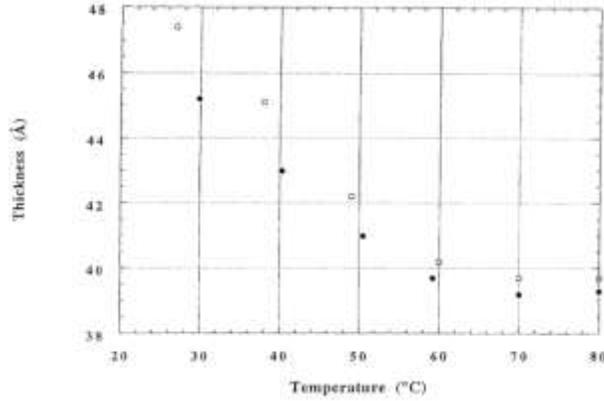
**Figure 0-4** Reproducibility of the observed contraction phenomenon, An ultrathin PS film was annealed and then subsequently heated incrementally to 80°C cooled, and reheated to 80°C. (●) the first heating cycle and (○) the second heating cycle. [11]
