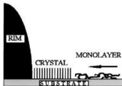
Figure 0-6 Model for crystallization of polymer mono-layer. [21]
