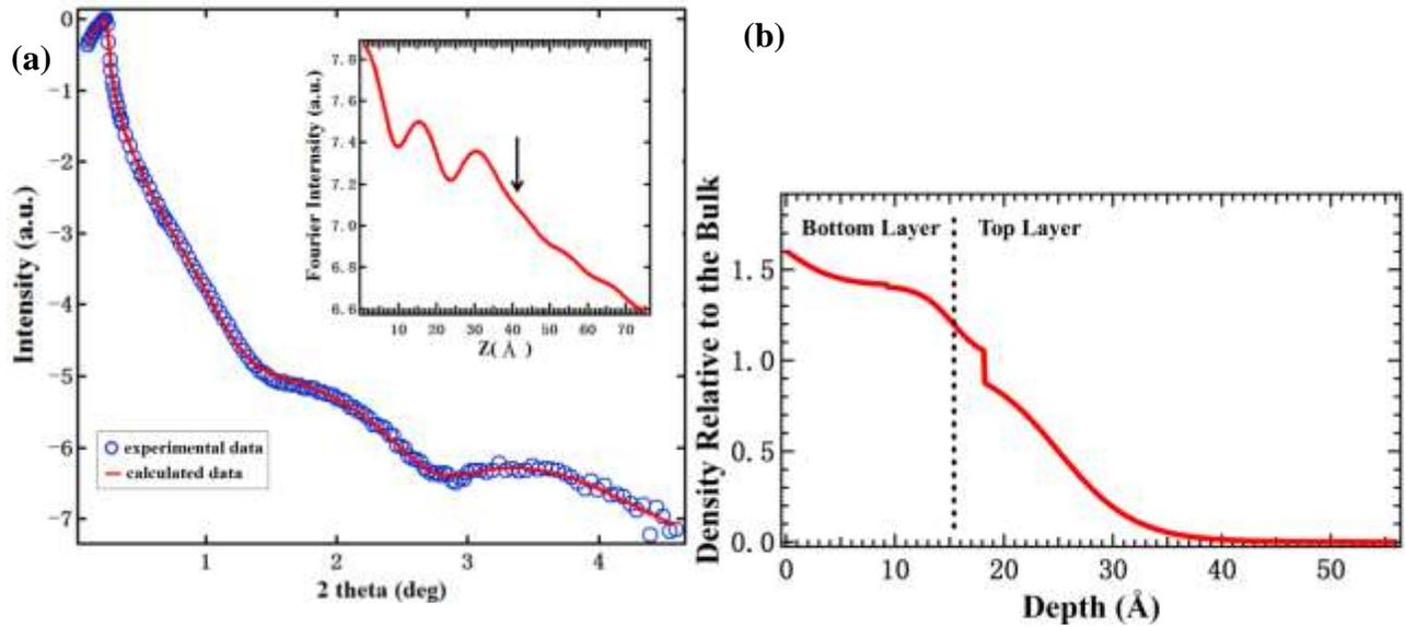
**Figure 3-3 (a)** Representative x-ray reflectivity profile for the PEO adsorbed layer is shown as symbols with best fittings as lines for the films. FT profile is interted . **(b)** Adsorbed layer density relative to the bulk.
