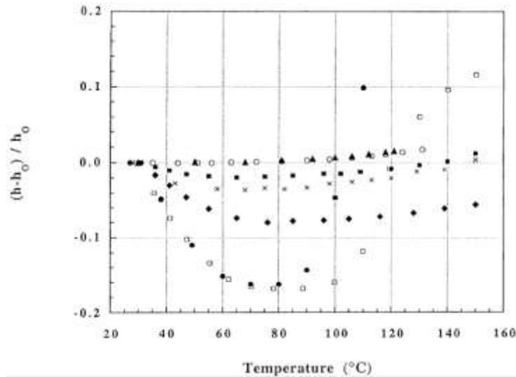
**Figure 0-5** Relative change in thickness of PS (Mw=573000) films on Si as a function of temperature.  $h_0$  is the initial thickness.  $h_0$  are denoted as (●)47.4Å, (□)49.9Å, (◆)100.4Å, (X) 155.1Å, (■)216.6Å, (○)264.3Å, (▲)833Å [11]
