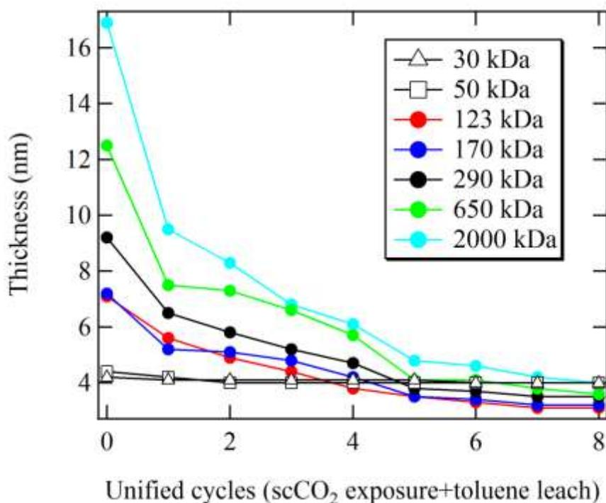
Figure 3-9 Plot of PS adsorbed layer thickness as a function of scCO<sub>2</sub> –toluene wash cycles\*
