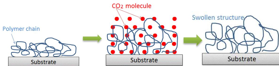
**Figure 0-8 Schematic concept of the scCO<sub>2</sub> –based processing polymer thin films.**
