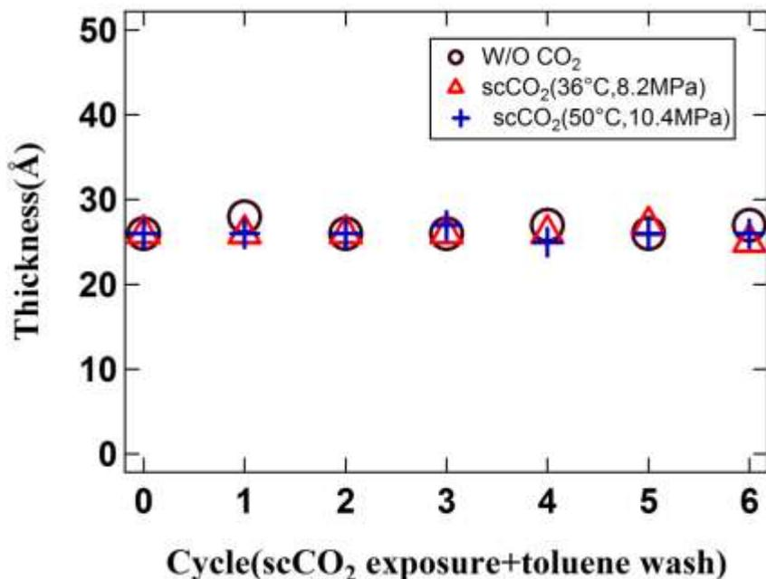
**Figure 3-10 Plot of PEO adsorbed layer thickness as a function of scCO<sub>2</sub> –toluene wash cycles**
