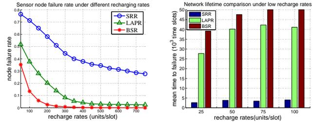
Fig. 6. Node failure rate and network lifetime. (a) Sensor node failure rate under different recharging rates. (b) Network lifetime comparison under low recharge rates from 25 to 100 (units/slot).
