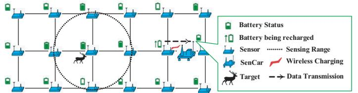
Fig. 1. System architecture of the wireless rechargeable sensor network.
