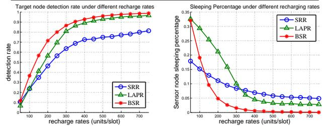
Fig. 4. Detection rate and sleeping percentage. (a) Target node detection rate under different recharge rates. (b) Sleeping percentage under different recharge rates.
