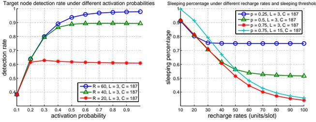
Fig. 3. Detection rate and sleeping probability of a 100-node sensor network. (a) Detection rate under different sensor activation probabilities. (b) Sleeping probability under different recharging rates and sleeping thresholds.
