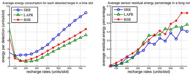
Fig. 5. Average node energy consumption per target detection and sensor residual energy in a long run (a) Average energy consumption for each detected target in a time slot (b) Average sensor residual energy percentage in a long run.
