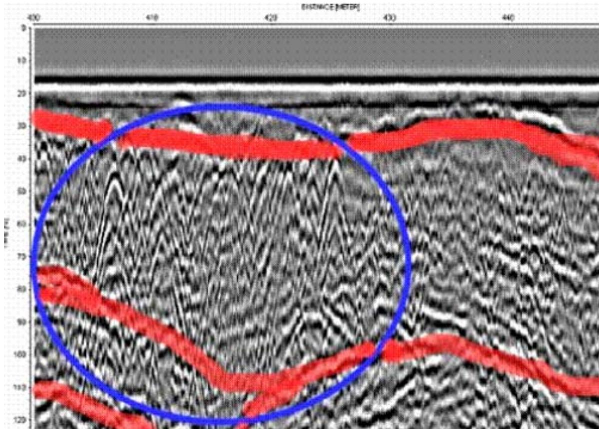
**Figure 3. Radargram from GPR line conducted with 200 MHz antenna. Boulder clump circled in blue. Boulders indicated by hyperbolas. Areas highlighted in red indicate boundaries of till-capping layer.**
