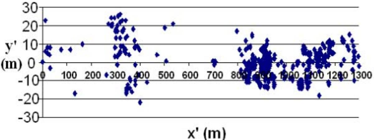
**Figure 2. Plot showing positions of boulders along the shoreline at Wildwood State Park. X' axis is distance along the beach (parallel to shoreline, y' axis is normal distance (perpendicular to shoreline). Exaggeration is roughly 6:1 in the y' axis direction.**
