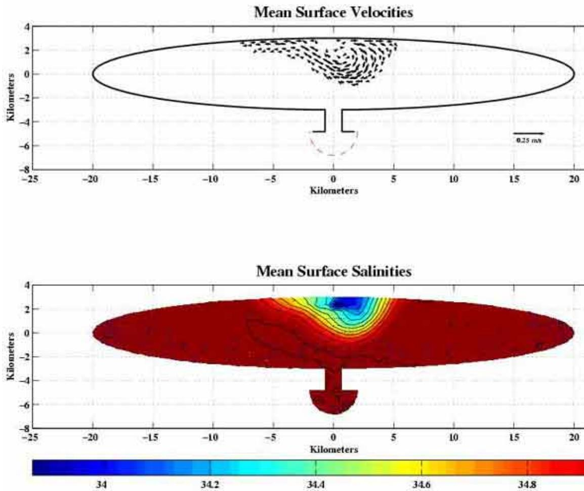
Figure 1. Surface velocities and salinities from a developing plume of low salinity water from a single area of submerged freshwater discharge.
