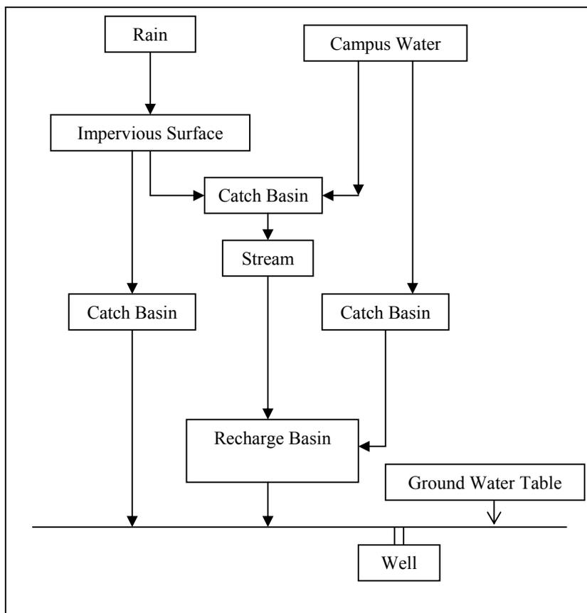
Figure 3. Flow chart of the sources and paths of water on campus. Campus water includes untreated cooling water and leaking chilled and hot water.
