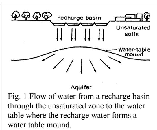
Fig. 1 Flow of water from a recharge basin through the unsaturated zone to the water table where the recharge water forms a water table mound.
