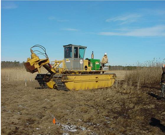
Figure 4 - Quality ditcher modified with “low-ground pressure” tracks. Environmental monitor on deck assessing environmental impact during operation.
