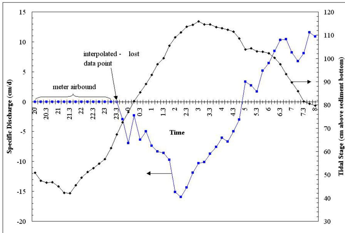
**Figure 3** Data set depicting the ability of the ultrasonic seepage meter to collect data in intertidal areas.
