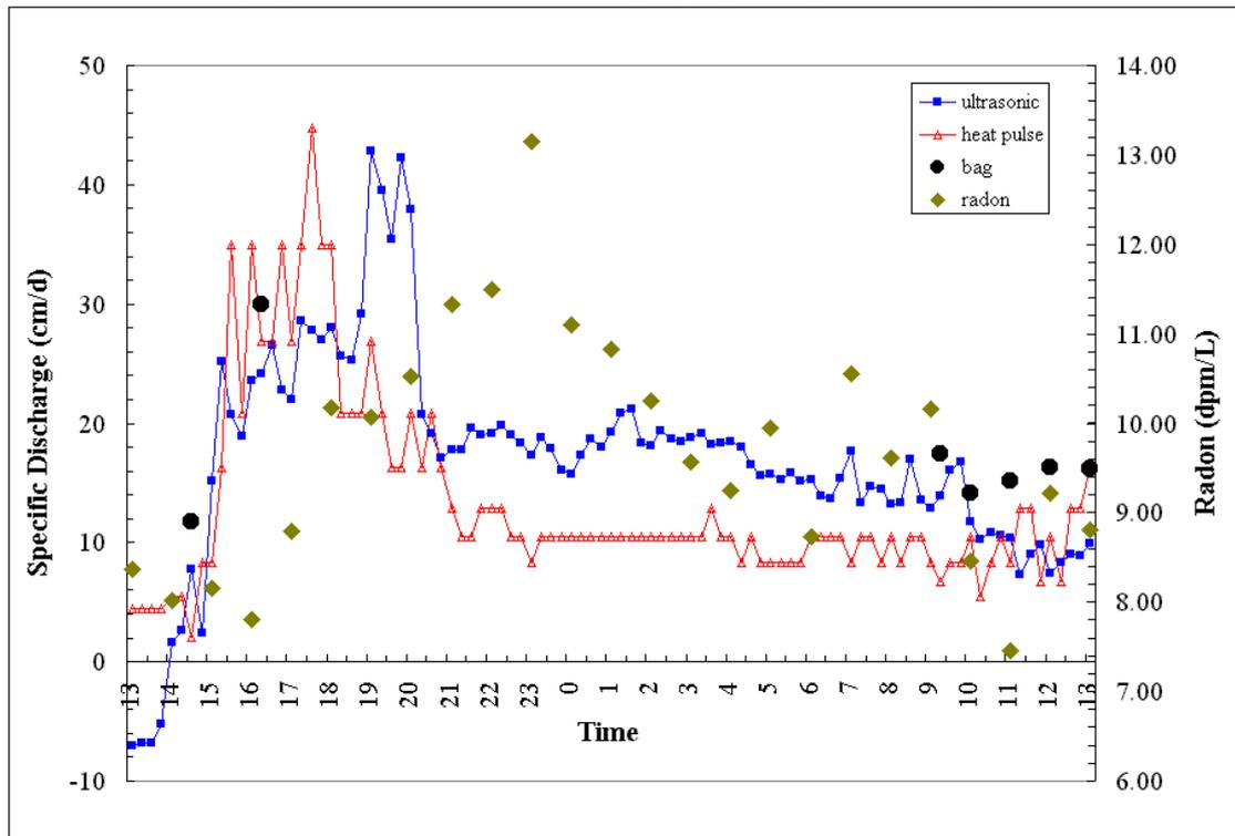
**Figure 2** Data set comparing preliminary SGD measurements at one station along a seepage transect (radon and manual measurements, Burnett, 2001; heat pulse data, Taniguchi, 2001).
