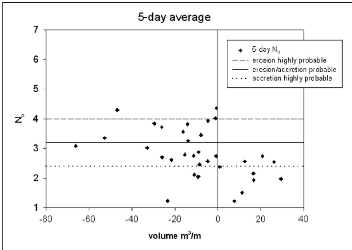
Figure 3. Kraus et al (1991) criteria applied to Dean number values calculated for wave parameters 5 days prior to profile measurements.
