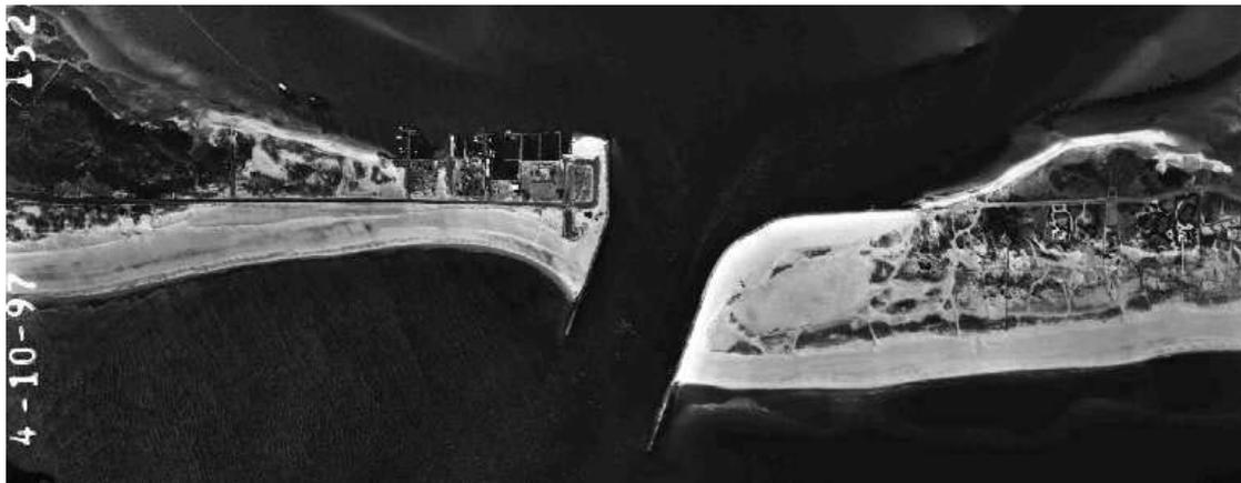
Figure 1. Shinnecock Inlet shoreline on 4/10/97. Shoreline appears in nourished state (fill placed on 1/97).
