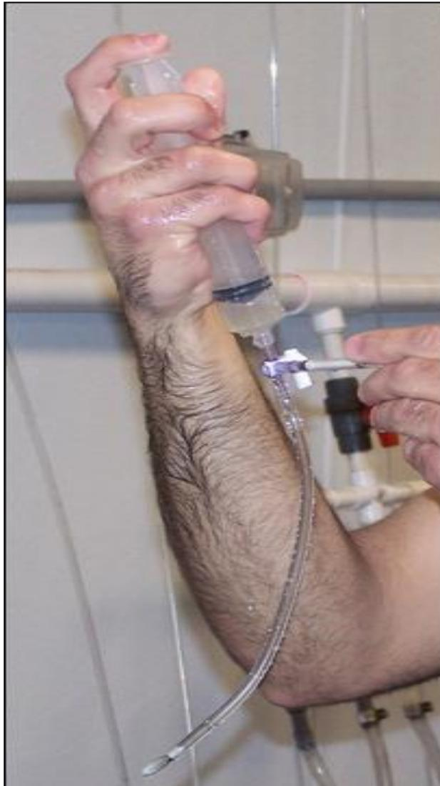
**Figure 4.** Porewater injection and sampling device.
