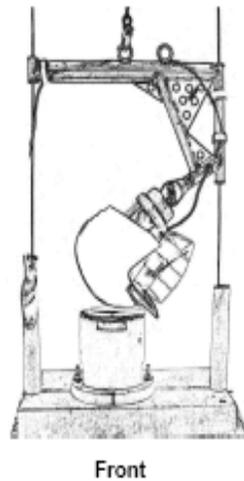
Figure 5. Helmet on head form mounted to drop test apparatus for frontal impact test. (NOCSAE DOC 041-04m04b)
