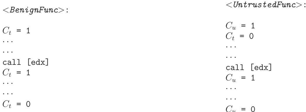
Figure 2.2: Scheme showing the points at which context flag bits are set and reset in a trusted function BenignFunc and an untrusted function UntrustedFunc . If only C_t is set, the program is in trusted context. If only C_u is set, the program is in untrusted context. If both bits are set, the program runs in trusted context on behalf of the untrusted code.
