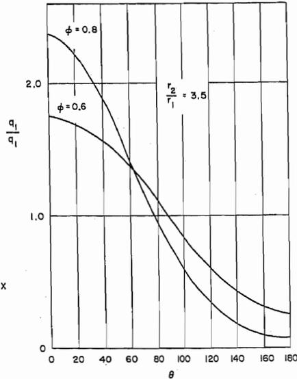
Fig. 2. Local heat flux on inner tube surface.
