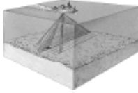
Figure 1: Cartoon of a multibeam system showing how the echo-sounding beams are formed by a combination of transmit and receive beam patterns.
